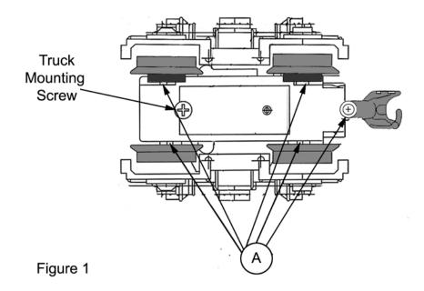
1. For the axles and coupler pivot points **Marked A**, we recommend that you lubricate with a small amount of light oil such as Bachmann E-Z Lube® #99984 Light Gear Oil. **Do not over-lubricate**.
